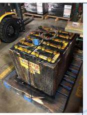
Improper battery maintenance can cause a littany of problems; from the obvious issues of ruining the battery or short run times to forklift operating issues such as coding out due to low voltage.
